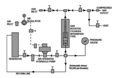
The Model GB-30 Gas Booster is rated for use up to 30,000 psi and has a 1:1 ratio. Displacement per stroke is 112 cubic inches.
